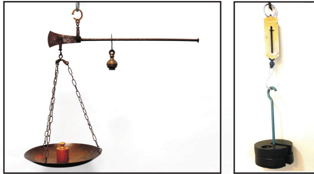
Figure 37. A steelyard based on rigid lever principle (left) and a spring balance based on deformation (right).
