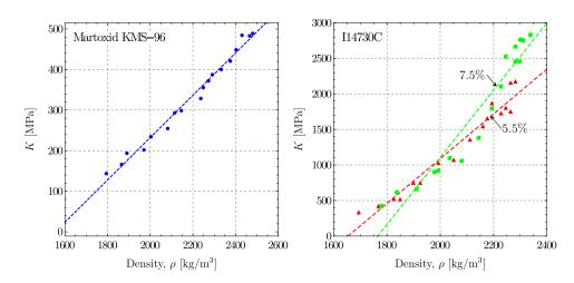
Figure 14: The elastic bulk modulus K as a function of the green's density for the Martoxid KMS-96 powder (left) and the I14730C powder at 5.5% (red/triangular spots) and 7.5% (green/square spots) water content (right).
