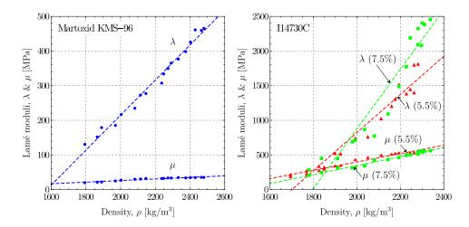
Figure 13: The Lamé elastic constants  $\lambda$  and  $\mu$  as functions of the green's density for the Martoxid KMS-96 powder (left) and the I14730C powder at 5.5% (red/triangular spots) and 7.5% (green/square spots) water content (right).
