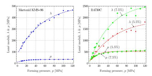
Figure 9: Variation of the elastic Lamé constants  $\lambda$  and  $\mu$  with the forming pressure for the Martoxid KMS-96 powder (left) and for the I14730C powder at 5.5% (red/triangular spots) and 7.5% (green/square spots) water content (right).
