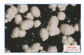
Figure 2: Micrograph of the Martoxid KMS-96 powder (left) and of the I14730C powder at 5.5% water content (right). The photos have been taken with a Nikon SMZ-800 optical microscope equipped with DSF1i camera head. The scale bar is 200 µm.
