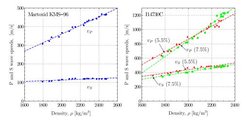
Figure 11: Propagation speed of pressure waves and shear waves as a function of the green's density for the Martoxid KMS-96 powder (left) and the I14730C powder at 5.5% (red/triangular spots) and 7.5% (green/square spots) water content (right).
