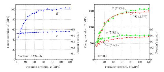
Figure 8: Variation of the Young modulus E and of the Poisson's ratio  $\nu$  with the forming pressure for the Martoxid KMS-96 powder (left) and for the I14730C powder at 5.5% (red/triangular spots) and 7.5% (green/square spots) water content (right).
