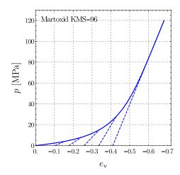
**Figure 16:** Predicted isostatic forming response at increasing pressure p, with unloading for an alumina powder (Martoxid KMS-96). Note the progressive increase in stiffness of the elastic response (visible at unloading), due to elastoplastic coupling.
