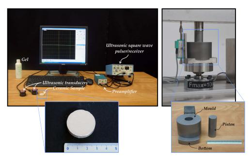
Figure 3: The experimental set up for ultrasonic testing.
