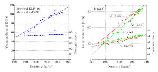
Figure 12: The elastic Young modulus E and the Poisson's ratio  $\nu$  as functions of the green's density for the Martoxid KMS-96 powder (left) and the I14730C powder at 5.5% (red/triangular spots) and 7.5% (green/square spots) water content (right).
