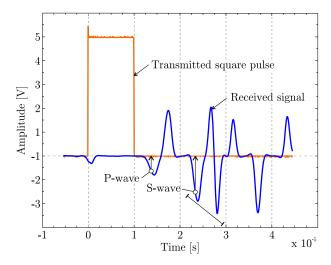
Figure 4: An example of filtered signal obtained using two normal incidence shear wave transducers. The signal was measured by a the Digitizer/Oscilloscope and analysed in Matlab®. The transmitted square wave is reported in red and the received wave-form is reported in blue.
