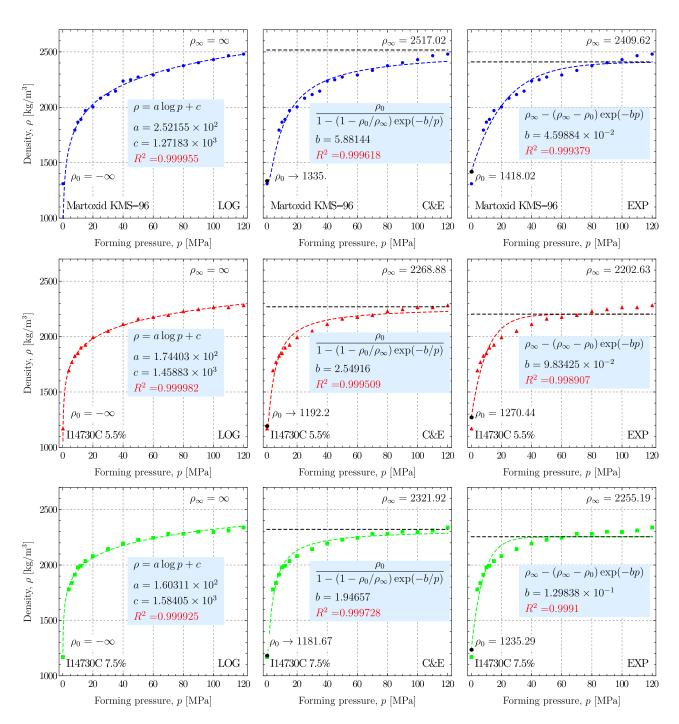
Figure 6: Fitting laws for the compaction behaviour of the Martoxid KMS-96 (upper part), of the I14730C at w=5.5% (central part) and at w=7.5% (lower part) powders. From left to right: Logarithmic law (2) ('LOG'); Cooper and Eaton law (3) ('C&E'); Exponential law (4) ('EXP').  $R^2$  denotes the coefficient of determination.
