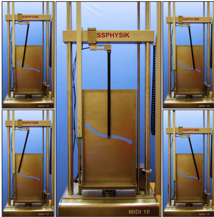
Fig. 6: Experimental set-up for the structure providing the neutral postcritical response. Two photos taken during elongation (shortening) are reported on the left (on the right).
