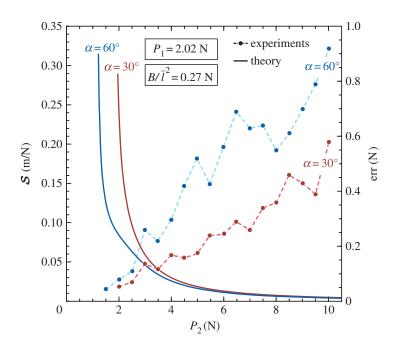
**Figure 5.** Sensitivity (denoted by S) of the deformable arm scale (at two inclinations  $\alpha$ ) as a function of the load  $P_2$ , reported together with the maximum absolute error (denoted by 'err') on the loads measured on the prototype shown in figure 1*a*. (Online version in colour.)
