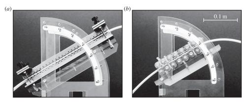
Figure 3. Two prototypes of the deformable arm scale: (a) prototype 0 and (b) prototype 1.
