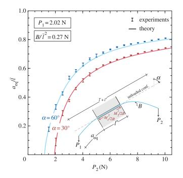
**Figure 4.** Equilibrium length  $a_{eq}$  measured on prototype 1 shown in figure 1*a* (at two inclinations  $\alpha$ ) for different loads  $P_2$  versus theoretical predictions. (Online version in colour.)
