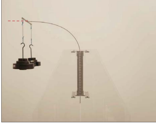
Figure 4.6: The vertical and upward Eshelby-like force (equal and opposite to the applied downward load) generated by the sliding sleeve makes the equilibrium configuration possible, even if unstable. Note that the tangent to the end of the blade is horizontal, as will be theoretically rationalized in Sect. 4.2.
