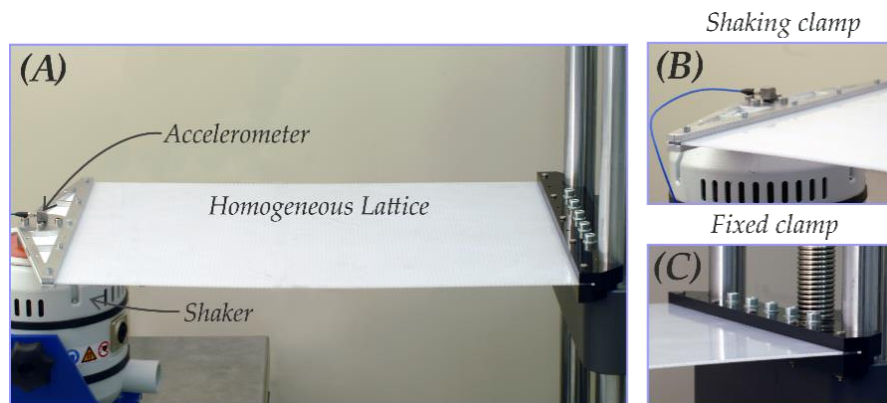
Figure 3: (A) The experimental setup employed in the cymatic experiments. A thin transparent film was used to cover the flexural lattice system to enable the use of powder for the Hooke-Chladni-Faraday visualization; (B) and (C) The detail of the shaking clamp and the fixed clamp respectively.
