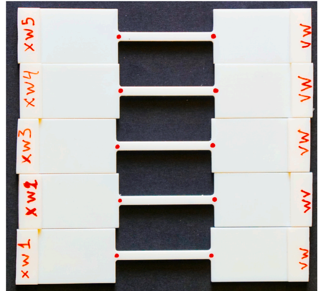
Fig. 18. The fabricated dog-bone samples uni-axially tested to estimate the mechanical properties of the bulk material (Vero PureWhite™) used to print the FG lattice structures.
