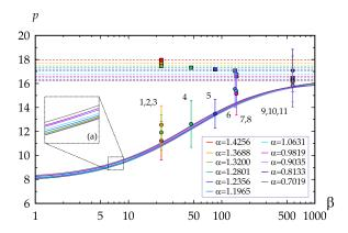
FIG. 9. Solid curves mark the critical flutter load versus damping ratio  $\beta=\gamma/\eta$  at different values of mass ratio  $\alpha$  and corresponding fixed values of  $\eta$ , see Table I. The experimental data are shown by spots with error bars. Dashed lines indicate the critical flutter load of the undamped Pflüger column for the same values of  $\alpha$ .
