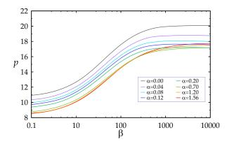
FIG. 5. Each curve, computed with the use of the equation (23), shows the critical flutter load in the limit of vanishing dissipation as a function of the damping ratio  $\beta$  for the discretized model with N=2 and  $\chi=1$  and corresponds to a different mass ratio  $\alpha$  (reported in the legend). Note that at large mass ratios  $0.7 \lesssim \alpha \leq \pi/2$  the curves form a dense family.
