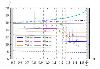
FIG. 8. Critical flutter load p versus mass ratio  $\alpha$ . Theoretical predictions based on Eq. (7) are plotted (the upper dashed curve) when damping is absent, when only external ( $\gamma$ , dot-dashed lines) or internal ( $\eta$ , lower dashed lines) damping is present, and (solid lines) when both damping mechanisms are present. Experimental results are marked by diamonds with error bars. The tested samples are numerated and their characteristics reported in Table I.
