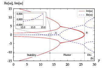
FIG. 7. Pulsation (red solid curves) and growth rates (blue dashed curves) for the Pflüger column versus the dimensionless load p (a) without damping and (b) in the presence of a Kelvin-Voigt damping for the material  $(\eta)$  and air drag  $(\gamma)$ , demonstrating the drop in the onset of flutter. The plots were obtained with the parameters representative of sample 5 in Table I.
