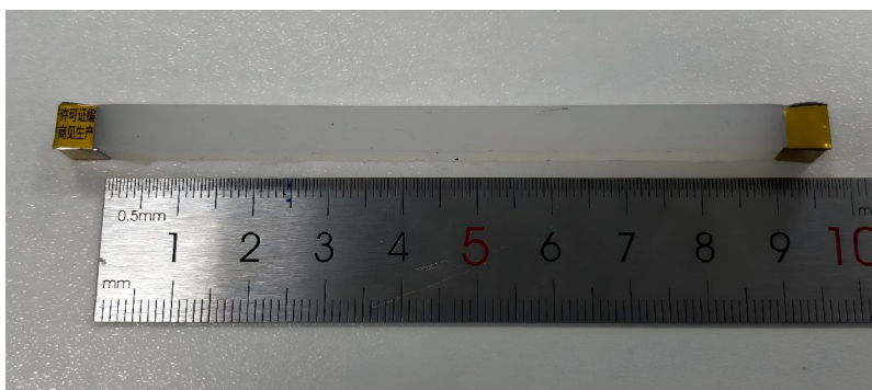
Fig. S8. Photograph of the test sample used for the cantilever beam resonance method.
